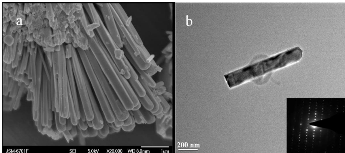
**Figure 2.** Morphology and structure of the as-prepared Sb<sub>2</sub>S<sub>3</sub> material characterised by **a** - FESEM and **b** - TEM
