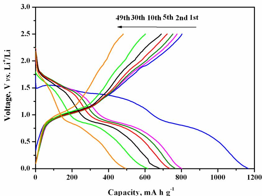
**Figure 5.** Potential profiles of the as-prepared Sb<sub>2</sub>S<sub>3</sub> sample in cycles 1, 2, 5, 10, 30 and 49 at a current density of 100 mA g<sup>-1</sup>
