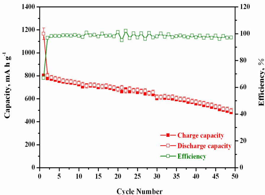
**Fig. 6.** Cycle performance of the as-prepared Sb<sub>2</sub>S<sub>3</sub> material at a current density of 100 mA·g<sup>-1</sup>.
