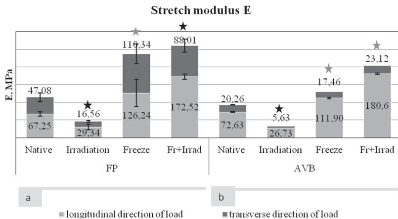
**Figure 2.** Stretch modulus (*E*) in longitudinal and transverse directions of fibers: *a* – FP, *b* – AVL; ★ – differences are statistically significant if compared with control,  $p < 0,05$ .
