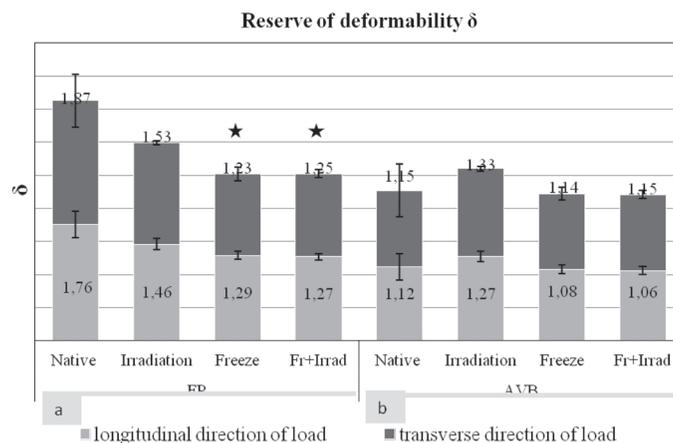
**Figure 5.** Reserve of deformability ( $\delta$ ) in longitudinal and transverse directions of fibers: a – FP, b – AVL; ★ – differences are statistically significant if compared with control,  $p < 0,05$ .
