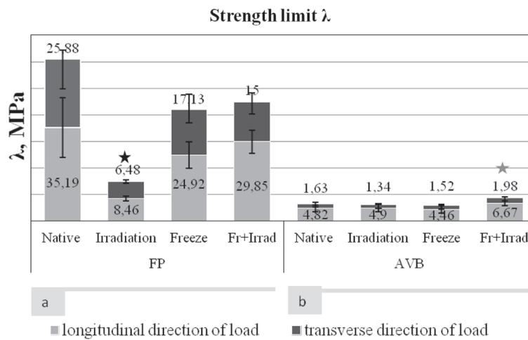
Figure 3. Strength limit ( $\lambda$ ) in longitudinal and transverse directions of fibers: a – FP, b – AVL; \* – differences are statistically significant if compared with control,  $p < 0,05$ .
