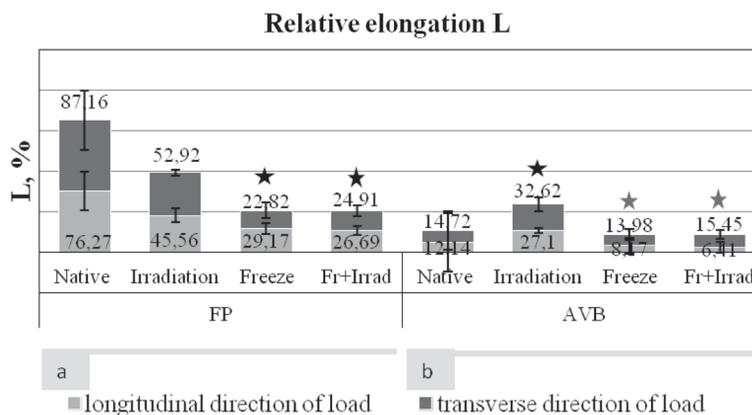
Figure 4. Relative elongation (L) in longitudinal and transverse directions of fibers: a – FP, b – AVL; \* – statistically significant if compared with control,  $p < 0,05$ .
