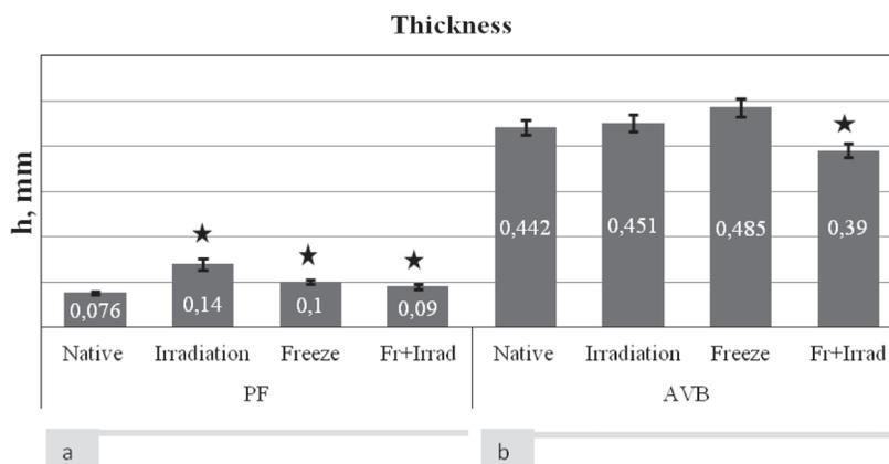
**Figure 1.** Thickness ( $h$ ) in longitudinal and transverse directions of fibers: a – FP, b – AVL; ★ – differences are statistically significant if compared with control,  $p < 0,05$ ,  $n=160$ .
