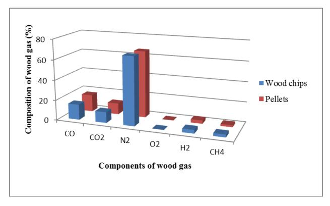
**Figure 1.** The wood gas composition from gasification wood chips and pellets **Slika 1.** Sastav drvnog plina proizveden rasplinjavanjem drvnih strugotina i peleta
