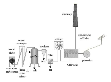
**Figure 2.** The scheme cogeneration device low-power to gasification of wood biomass **Slika 2.** Shema kogeneracijskog uređaja male snage na bazi rasplinjavanja drvne biomase
