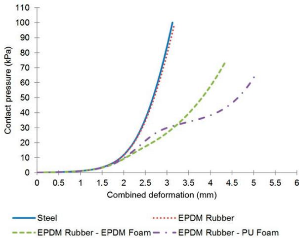
Figure 7 Contact pressure of the fingertip versus the vertical deformation of the fingertip and tool handle material combined [23]
