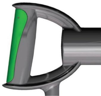
Figure 12 Virtual model of redesigned handle
