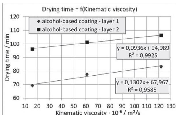
**Figure 4** Influence of the alcohol-based coating kinematic viscosity on its drying time. Sand grain size  $d_L = 0,24 \text{ mm}$ ,  $T = 22 \text{ }^\circ\text{C}$ ,  $W = 23 \%$
