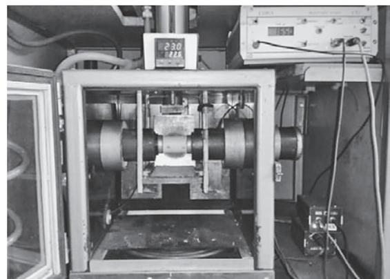
Figure 1 Stand for ultrasound investigations of the kinetics of the protective coatings drying process [14, 15]
