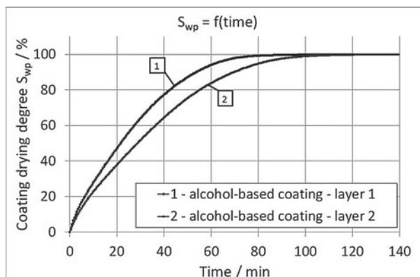
**Figure 2** Drying process of the alcohol-based protective coating. Kinematic viscosity of the coating  $\nu = 61 \cdot 10^{-6}$  m<sup>2</sup>/s, ambient temperature  $T = 22$  °C, air humidity  $W = 24$  %, immersion time  $t = 30$  s
