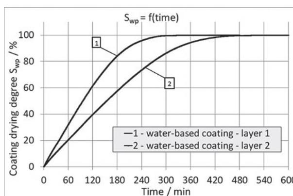
**Figure 3** Drying process of the water-based protective coating.  $\nu = 61 \cdot 10^{-6}$  m<sup>2</sup>/s,  $T = 22$  °C,  $W = 24$  %,  $t = 30$  s
