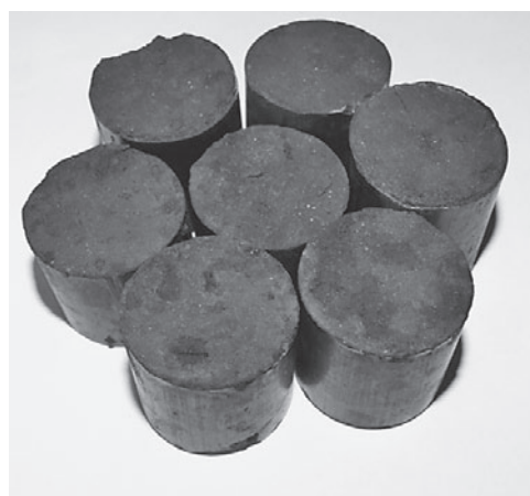
Figure 1 The obtained copper concentrate briquettes
