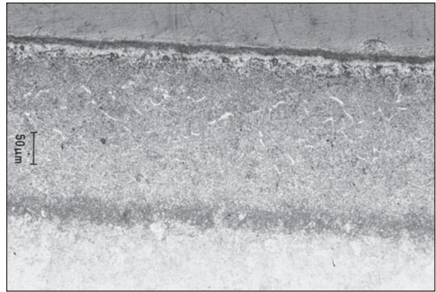
Figure 4 Steel 100Cr6 nitrided layer (D)
