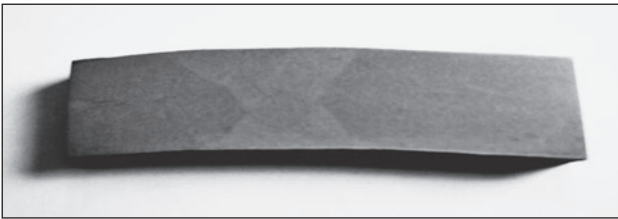
Figure 10 Cross-cut section of pipe wall with welding
