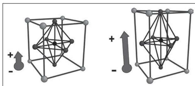
**Figure 1** Working principle of piezoelectric actuator
