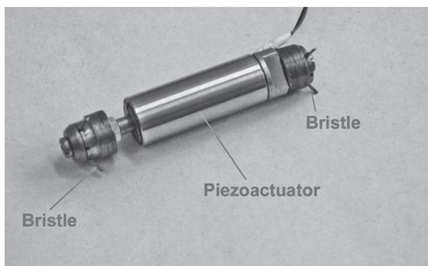
Figure 6 In-pipe robot with piezoactuator
