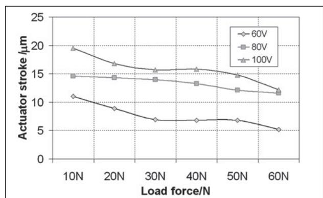
Figure 4 Measured characteristic of piezostack for different excitation voltages
