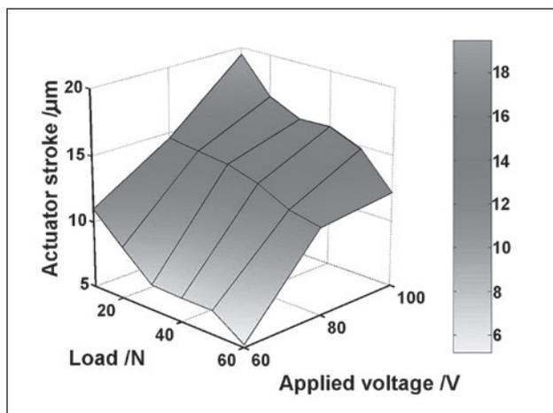
Figure 5 Measured characteristic of piezostack
