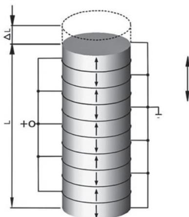
Figure 2 Piezostack structure [8]
