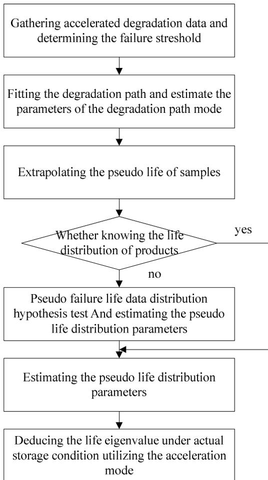
Figure 4. Photoelectric devices storage life assessing method flows based on pseudo life.
