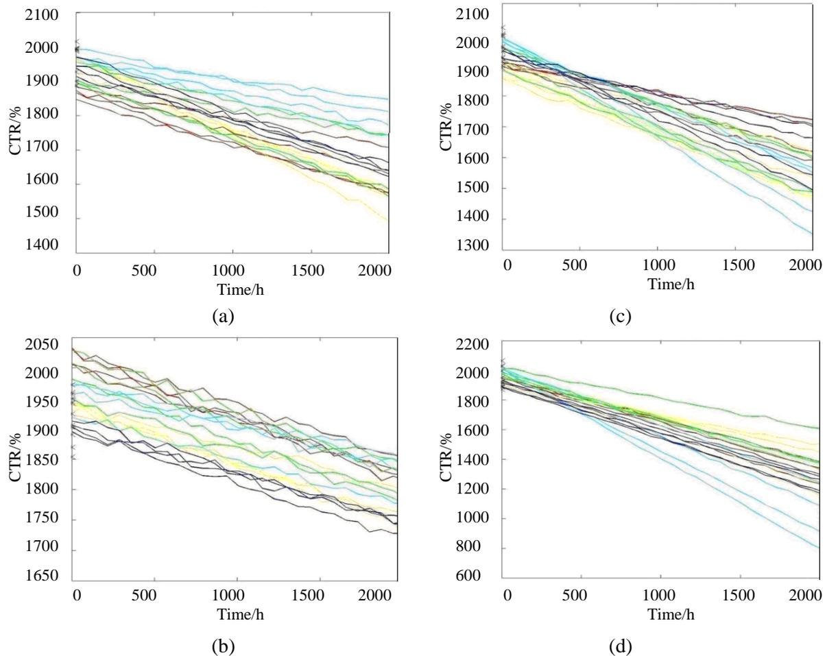
Figure 2. CTR degradation paths: (a) CTR degradation paths under 100, (b) CTR degradation paths under 125, (c) CTR degradation paths under 150, (d) CTR degradation paths under 175.
