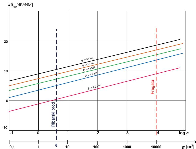
Figure 4. Diagram showing dependence of radar range on the reflective surface of the target for different radars 4
