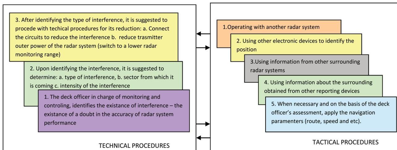
Figure 1. Procedures of the radar system operator in case of intentional jamming 4
