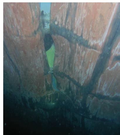
Slika 8. Oštećenja trupa s vanjske strane Figure 8. Damage to the hull from the outer side
