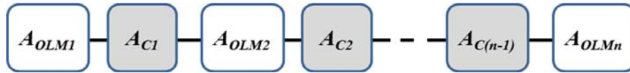
Fig. 5 Availability model for serial structure with n OLM elements and (n-1) cable sections
