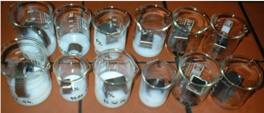
Figure 8: Corrosion examination on pipe samples in 1 % emulsion, immersed and coated only, without immersing
