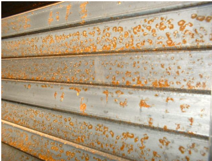
Figure 2: Corroded precise welded pipes 25 mm x 25 mm x 2 mm
