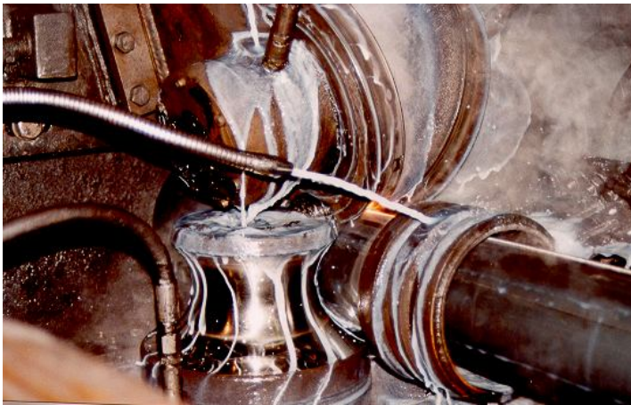
Figure 1: Cooling of an impeder with a cooling emulsion during pipe welding
