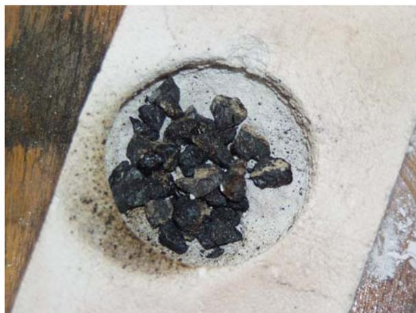
Figure 4. **Rock samples after the flame action**
