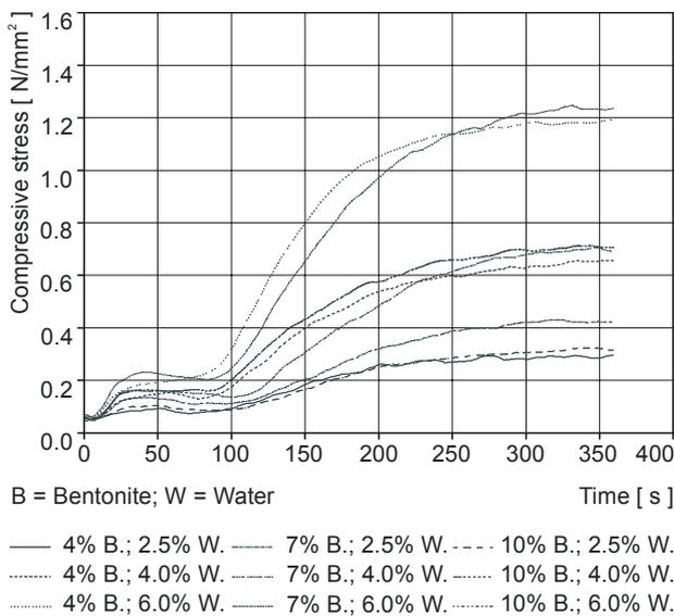
Figure 7. Graphical presentation of the measuring results for the mould mixture featuring granularity G3
