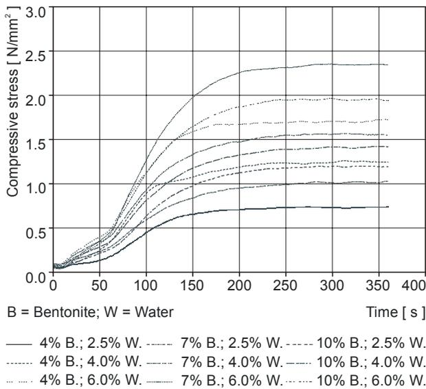
Figure 6. Graphical presentation of the measuring results for the mould mixture featuring granularity G2
