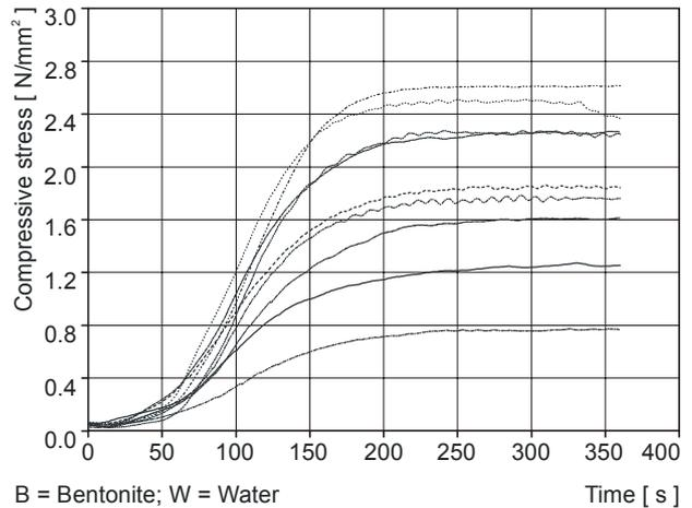
Figure 5. Graphical presentation of the measuring results for the mould mixture featuring granularity G1
