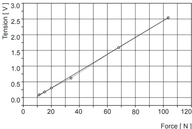
Figure 3. **Calibrating diagram of the modified design of the compressive stresses gauge**
