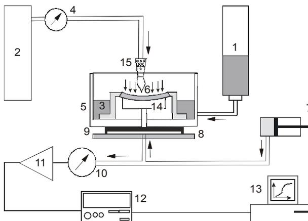
Figure 2. **The modified device for measuring compressive stresses.**
