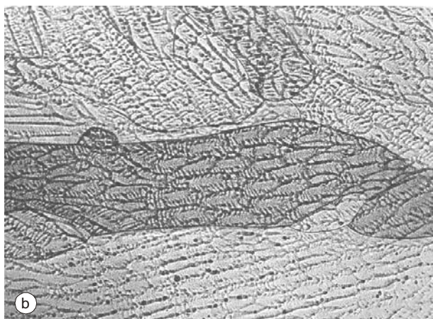
Figure 1. Microstructure of niobium alloy 10VMTs: a-base metal; b - welded joint. Optical microscopy. Magnification: a - x400, b - x200
