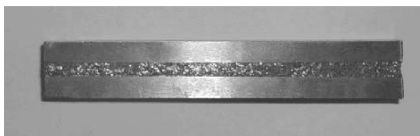
Figure 3. Three layer rod prepared from the bronze powder (surface layers) and bronze hollow spheres (central layer)
