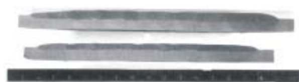
Figure 9. Macro specimens of the welds surfaced with a triple-wire electrode; d_w = 1.2 mm; I = 190 A/wire; U = 41 V, v_w = 0.3 m/min; b = 8 mm; L = 20 mm; electrode negative; above: 25 % overlapping; below: 50 % overlapping
