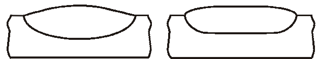
Figure 5. Shape of the surfacing weld as a function of the arrangement of wires of different diameters
