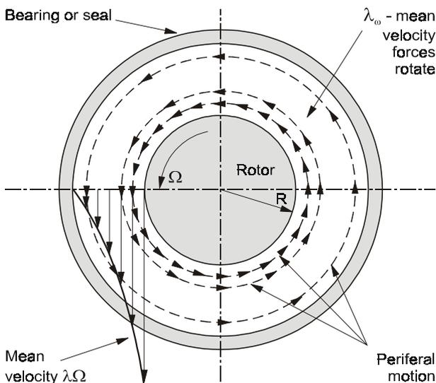
Figure 2. Profile speed fluid
