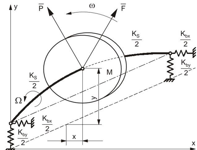
Figure 1. **Isotropy rotor system**
