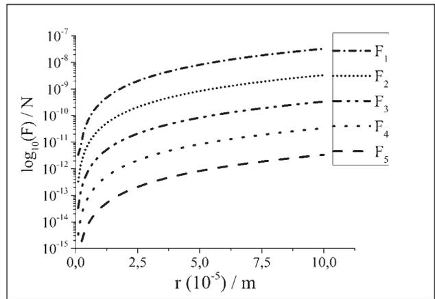
**Figure 3** The frictional force  $F_d$  for a single SiC particle in the vicinity of a vertical solidification front, which is advancing horizontally, for the particle velocities  $V_p = 10^{-5}$  /m s<sup>-1</sup> (ZnAl8/SiC<sub>p</sub>)
