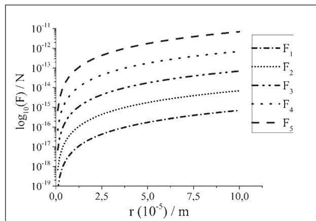
**Figure 8** The Saffman forces for ZA8/SiCp composite. ( $S=0,000001 / \text{m s}^{-1}$ )
