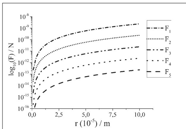
**Figure 5** The frictional force  $F_d$  for a single SiC particle in the vicinity of a vertical solidification front, which is advancing horizontally, for the particle velocities  $V_p = 10^{-6} / \text{m s}^{-1}$  (ZnAl27/SiC<sub>p</sub>)
