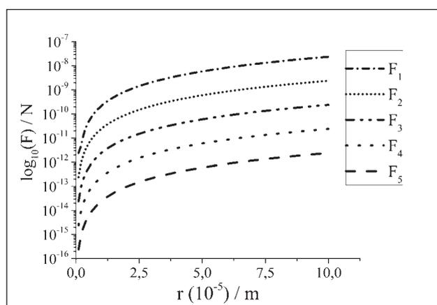
**Figure 6** The frictional force  $F_d$  for a single SiC particle in the vicinity of a vertical solidification front, which is advancing horizontally, for the particle velocities  $V_p = 10^{-5} / \text{m s}^{-1}$  (ZnAl27/SiC<sub>p</sub>)
