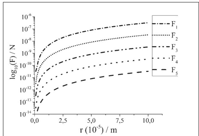
**Figure 4** The frictional force  $F_d$  for a single SiC particle in the vicinity of a vertical solidification front, which is advancing horizontally, for the particle velocities  $V_p = 10^{-4}$  /m s (ZnAl8/SiC<sub>p</sub>)
