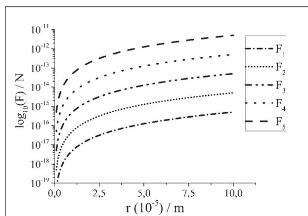
**Figure 9** The Saffman forces for ZA27/SiC<sub>p</sub> composite ( $S=0,000001 / \text{m s}^{-1}$ )
