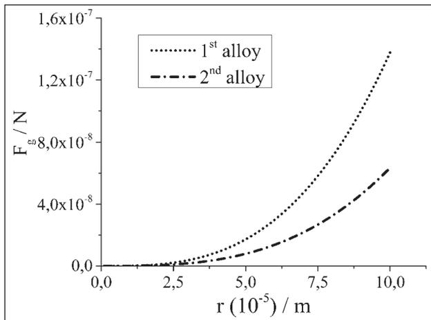
**Figure 1** The gravity force  $F_g$  against the SiC particle radius. 1st alloy denotes ZnAl8, 2nd alloy ZnAl27
