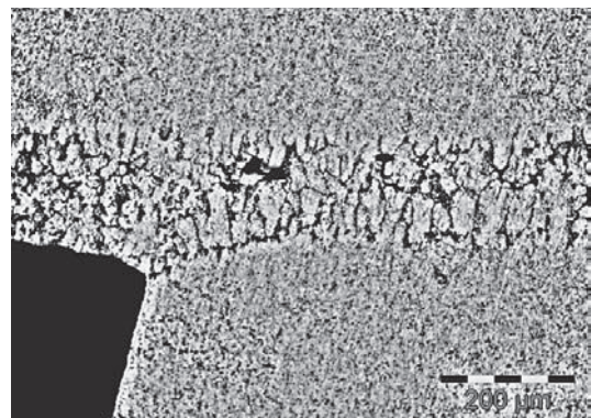
Figure 8 Technology No. 52: Technological process TP III AL for surfaces preparation, allowance material bed on a base material surface, A3 probe
