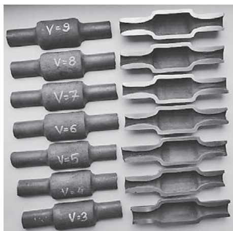
Figure 4 Products produced in the experimental investigations of the effect of linear velocity the rolls
