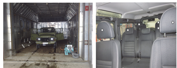
Figure 14 Hard Top in cold chamber and layout of sensors on the seats
