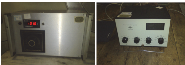
Figure 12 Thermal comfort meter 1212 B&K and Digital thermometer Omega 199
