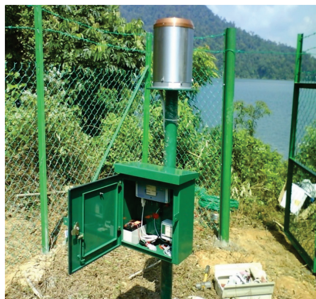
Figure 2 Tipping-bucket automatic recording equipment
