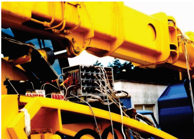
Figure 4 Data logging and processing equipment
