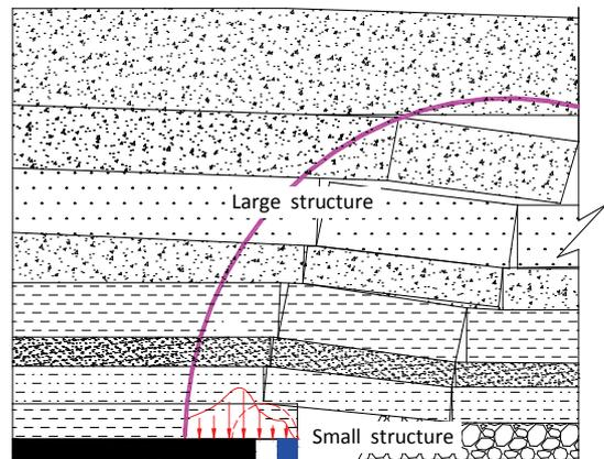
Figure 5 Mechanics model of "large/small structure" in mining without coal pillars
