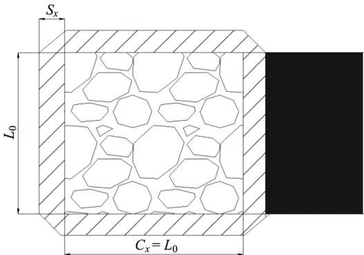
Figure 6 Diagram of abutment pressure range of distribution in stope digging
