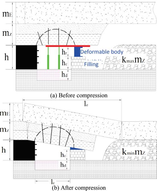
Figure 9 "Given deformation" mechanics structure
