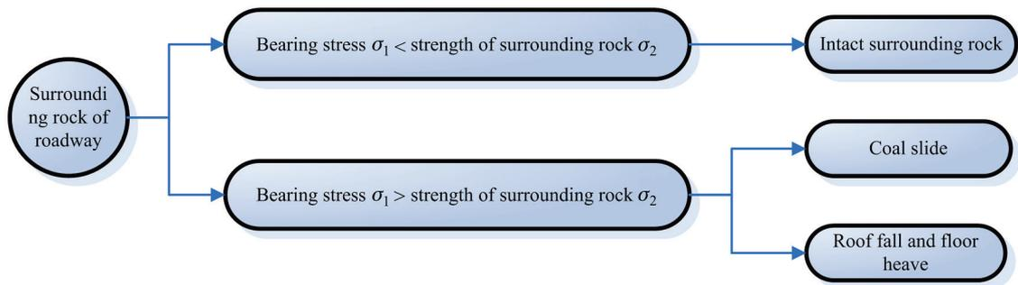
Figure 3 Causes of large deformation of roadway
