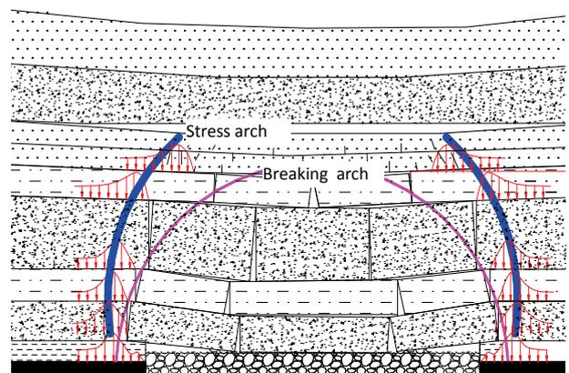
Figure 2 Schematic diagram of the "Double Arch Structure" model of a stope
