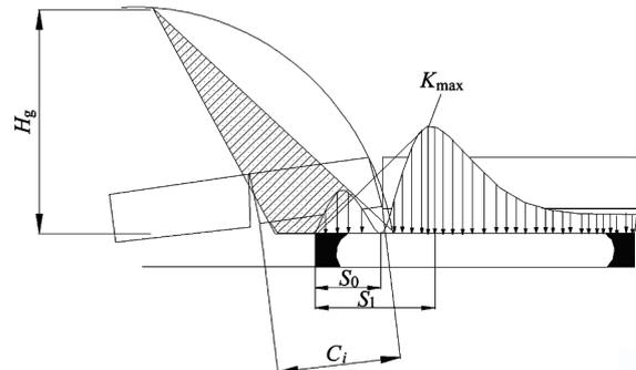
Figure 7 Calculation model for abutment pressure
