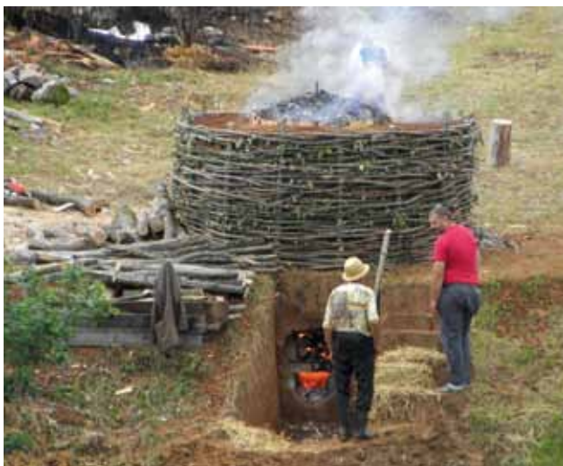
16 Paljenje vapnenice u selu Ponori (foto: T. Devčić) Igniting the limekiln in the village of Ponori (photo: T. Devčić)
