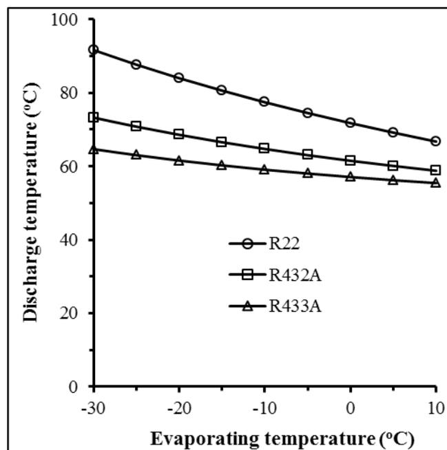
Fig. 7 Influence of the evaporating temperature on the discharge temperature
