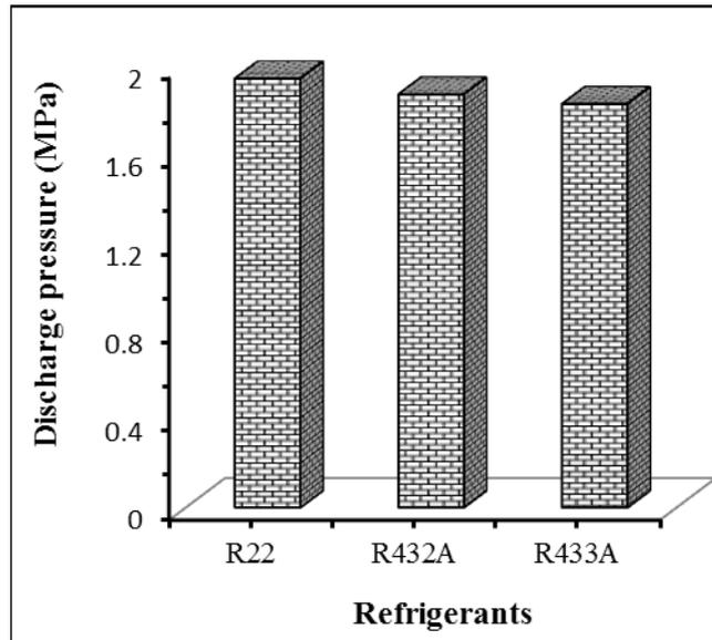
Fig. 8 Discharge pressure of the refrigerants at condensing temperature of 50°C
