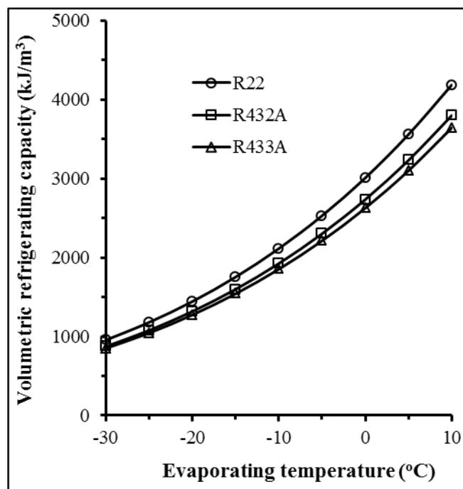
Fig. 9 Volumetric refrigerating capacity versus evaporator temperature
