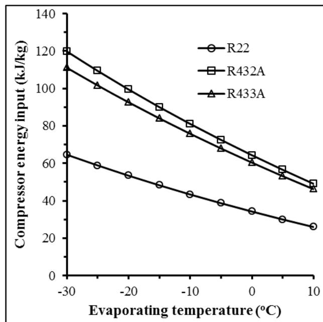
Fig. 4 Compressor energy input versus evaporating temperature
