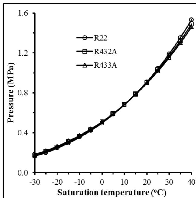
Fig. 2 Saturation vapour pressure curves
