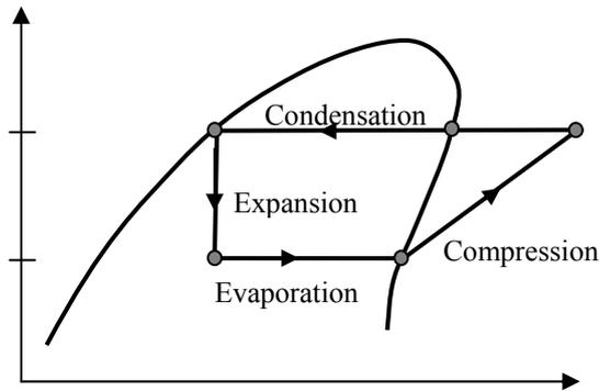
Fig. 1 Vapour compression refrigeration cycle on a p-h diagram
