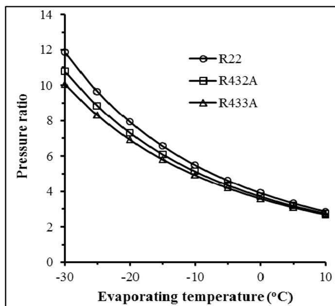
Fig. 6 Influence of the evaporating temperature on the pressure ratio
