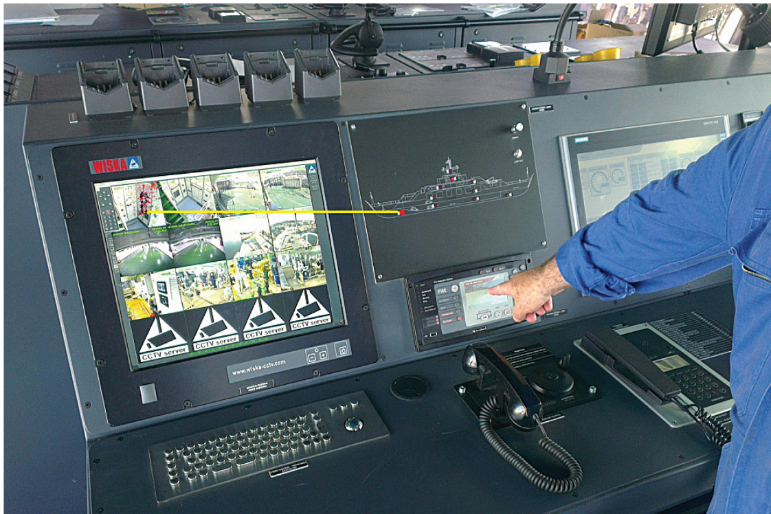
Figure 5 Display of connecting relations between CCTV video systems and fire detection alarm system on the Kornati - Jadrolinija ferryboat
