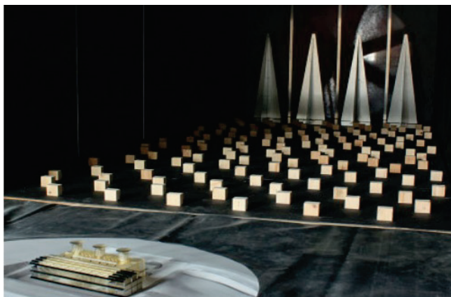
Figure 4 RATI Building model in the wind tunnel (with vortex generators and roughness elements) and the RPT model with the reference points
