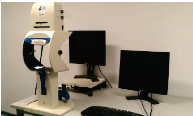
Figure 11 iView X Hi-speed eye movement tracking system
