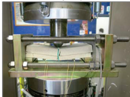
b) Double-layer plates rupture failure
