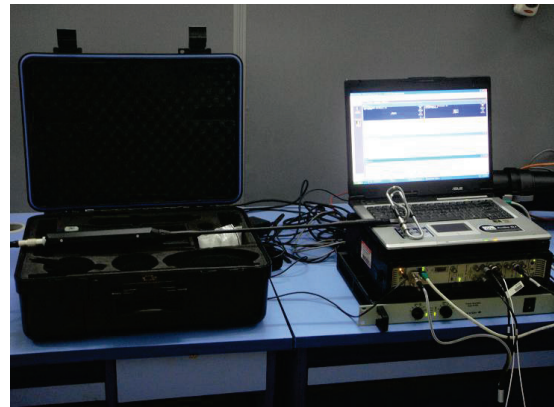
Figure 8 B&K3560 front end, power amplifier, notebook computer and sound intensity probe used in this experiment
