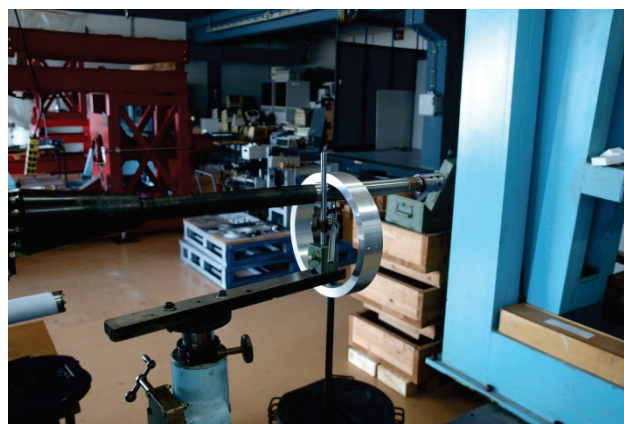
Figure 9 Sting deflection and slope measurement
