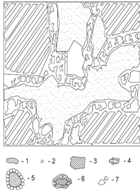
Figure 6 Structure of hardened mortar 1. Nonhydrated polymer-cement grains. 2. Polymer particles. 3. Fine aggregates and filling agent grains 4. The mixture of nonhydrated concrete particles and cement gel with residuum of polymer particles on their surface. 5. Mixture of cement gel and nonhydrated cement particles, tightly surrounded by polymer particles layer 6. Cement hydrates surrounded by polymeric films or membranes. 7. Entrained air.
