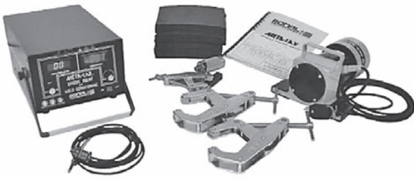
Figure 1 Equipment for residual stress relief by vibration [6]
