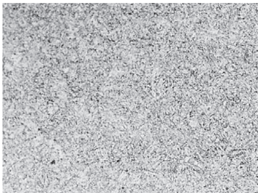
Figure 3 Base material structure P91 (magnified 200 x)
