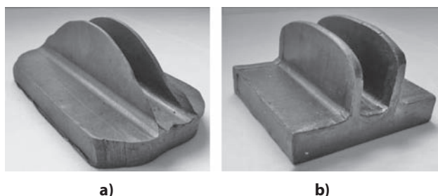
Figure 6 Shape of flat forgings with two ribs obtained in experimental research works for the process: a) semi-open die forging, b) closed-die forging
