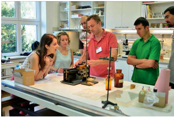
Figure 3 Microtoming the thin wood strips
