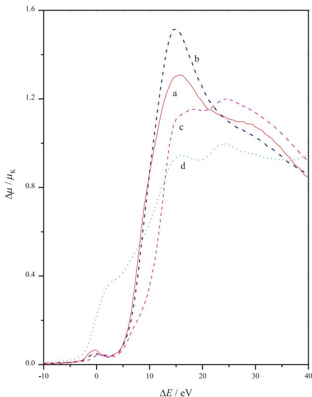
Figure 6. Normalised Co K-edge profiles of CoAlPO, as-synthesised (a); CoAlPO, rehydrated-calcined (b);  $[\text{Co}(\text{C}_2\text{H}_8\text{N}_2)_3]\text{Cl}_3 \cdot 4\text{H}_2\text{O}$  (c); Co, metal (d).
