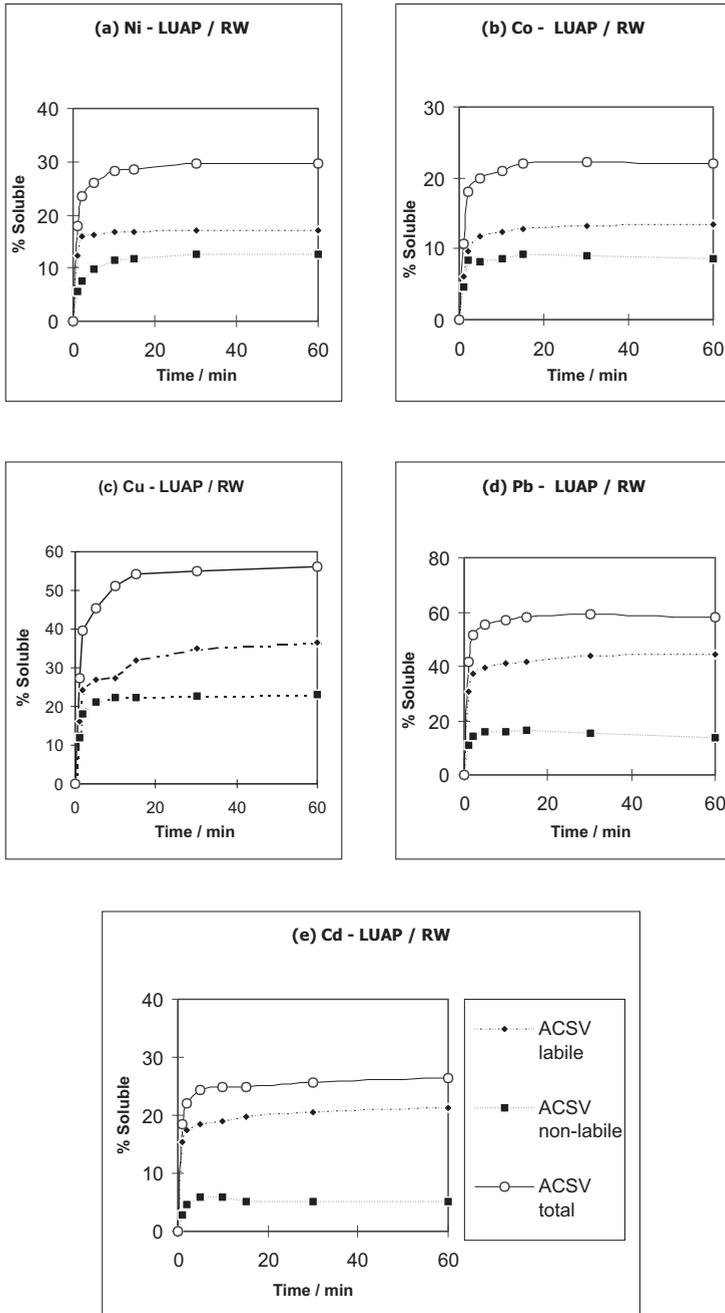
Figure 1. Release of trace metal fractions (ACSV<sub>non-labile</sub>, ACSV<sub>labile</sub> and total) from LUAP (10 mg l<sup>-1</sup>) into artificial rainwater (expressed as % soluble of total aerosol trace metal). (a) Ni, (b) Co, (c) Cu, (d) Pb, (e) Cd.
