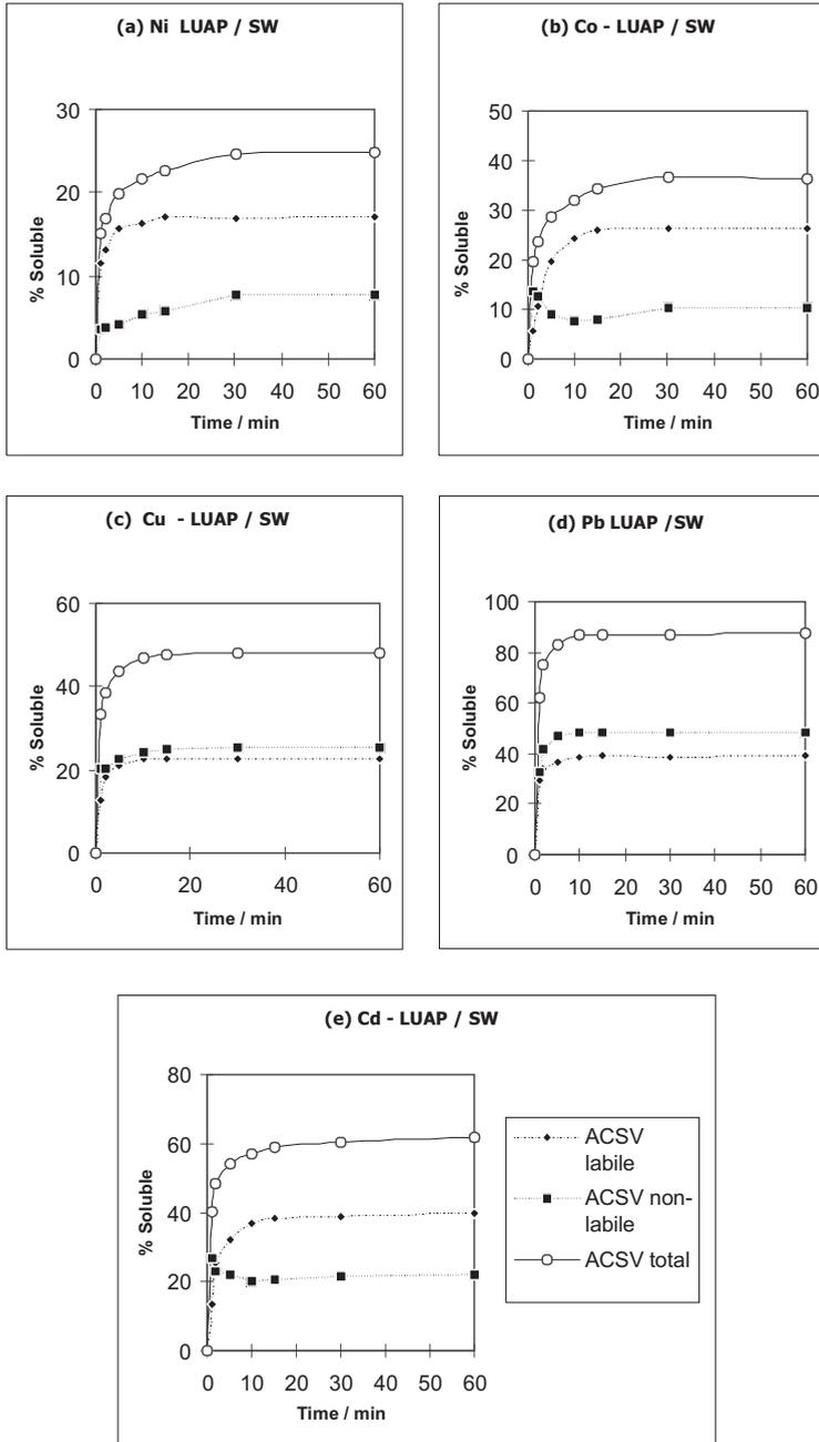
Figure 3. Release of trace metal fractions ( $ACSV_{non-labile}$ ,  $ACSV_{labile}$  and total) from LUAP ( $10 \text{ mg l}^{-1}$ ) into seawater (expressed as % soluble of total aerosol trace metal). (a) Ni, (b) Co, (c) Cu, (d) Pb, (e) Cd.
