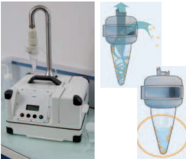
Figure 3.: Cyclonic air sampler (Coriolis Delta Air Sampler) as turbulent air flow pump
