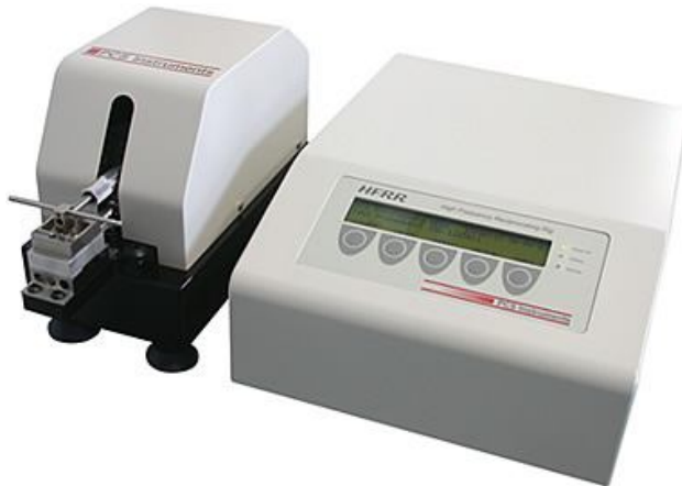
Figure 2: Standard test for diesel fuel lubricity - High Frequency Reciprocating Rig (HFRR) (Source: PCS instruments)
