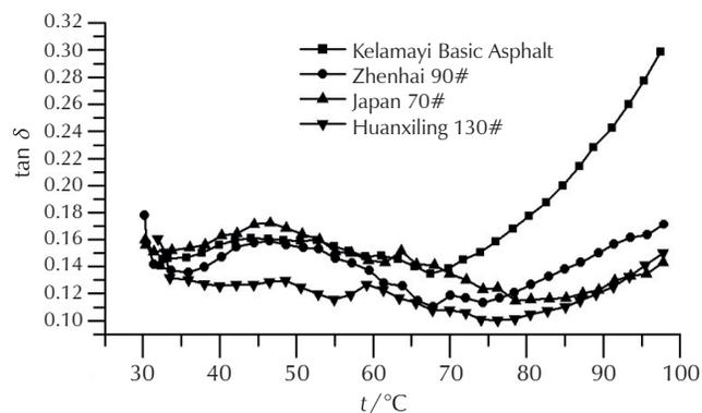
Fig. 3 – Temperature- $\tan \delta$  curve for different asphalts
