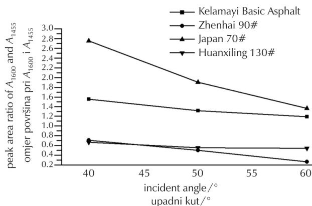
Fig. 1 – Benzene ring content ratio of different asphalts
