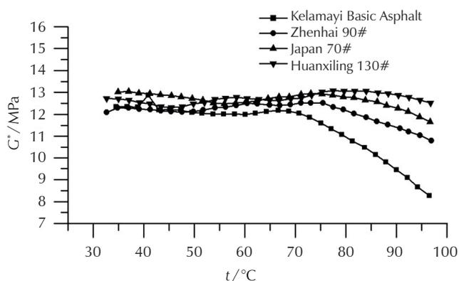
Fig. 2 – Temperature- $G^*$  curve for different asphalts
