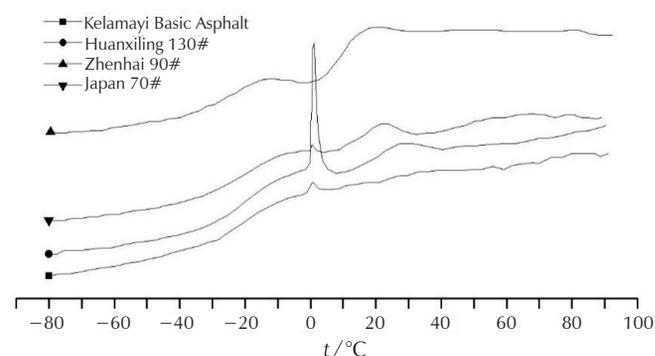
Fig. 4 – DSC curve of different original asphalts
