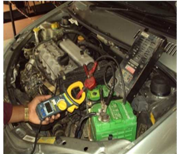
Fig. 1. Measurement of voltage dip and peak cranking current with old and new starter motor
