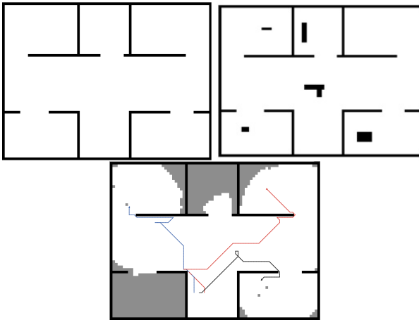
Fig. 2. The office-like environment used for testing the proposed exploration strategies without obstacles (left) and with some arbitrary obstacles (right) and a simulation snapshot for exploration with two robots (below).
