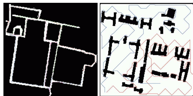
Fig. 7. The trajectories for the exploration strategy Stop-scan-replan-go after exploring the environment shown in Fig. 5 (left) and (middle).
