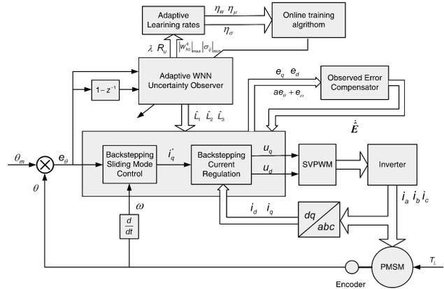
Fig. 2. Structure of proposed adaptive WNN backstepping sliding mode control system for PMSM drive
