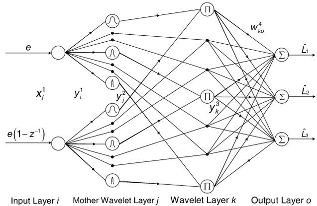
Fig. 1. Four-layer wavelet neural network
