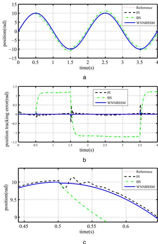
Fig. 4. Dynamic response of the PMSM drive system with uncertainties in Case2: (a) position tracking performance comparison of three controllers in Case2. (b) position tracking error of three controllers in Case2. (c) zoomed position tracking performance of three controllers at  $t = 0.5$  s
