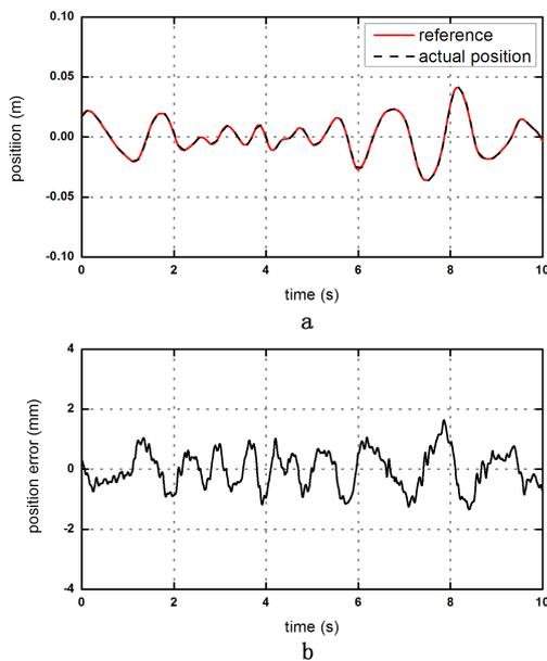
Fig. 8. Tracking performance and error on the command of the  $J$  spectral wave
