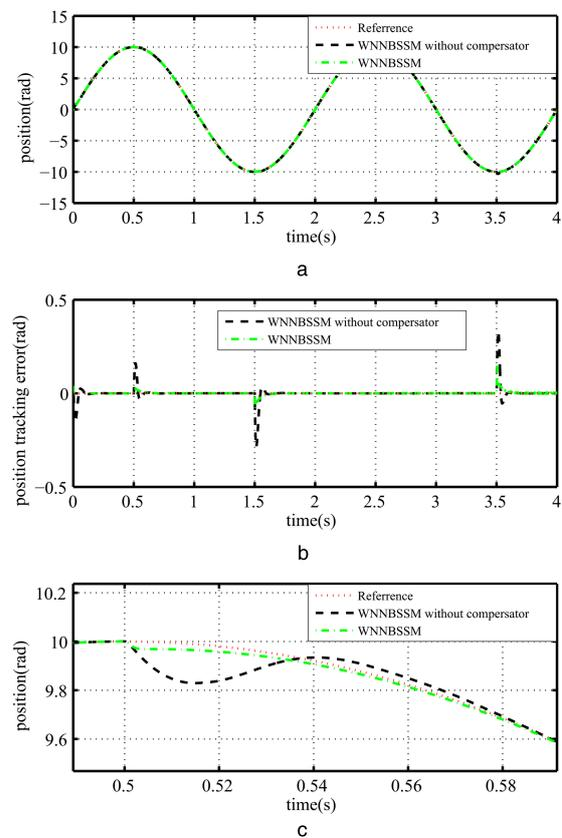
Fig. 5. Tracking response comparison for observed error compensator with uncertainties in Case2: (a) position tracking performance in Case2. (b) position tracking error in Case2. (c) zoomed position tracking performance at  $t = 0.5$  s
