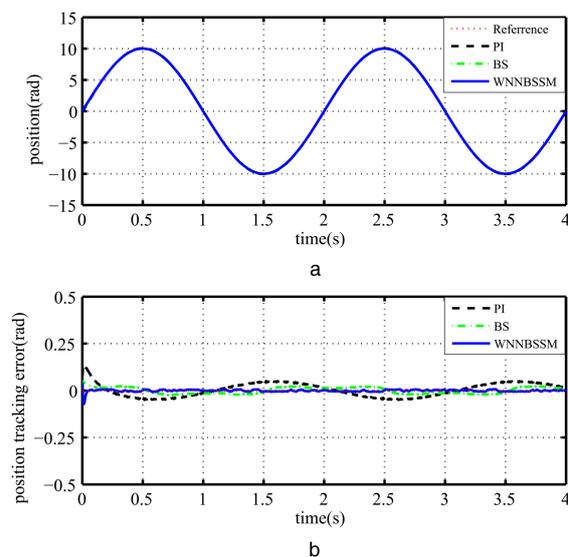
Fig. 3. Dynamic response of the PMSM drive system under nominal parameters: (a) position tracking performance for three controllers in Case1. (b) position tracking error for three controllers in Case1
