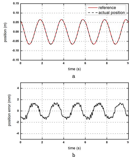
Fig. 7. Tracking performance and error on the command of the regular wave
