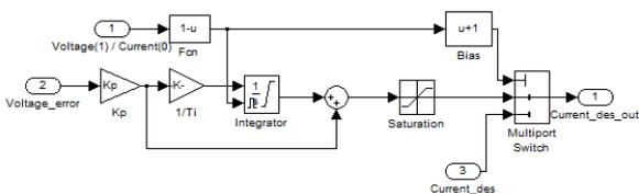
Fig. 8. Simulink model of voltage control algorithm
