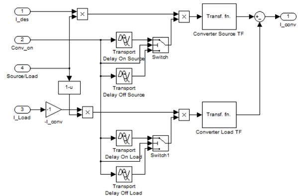
Fig. 5. Simulink model of bi-directional current controlled converter
