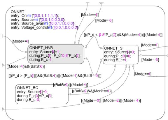
Fig. 12. Stateflow representation of the ONNET operation mode
