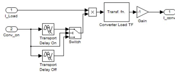
Fig. 7. Model of uni-directional (pure load) converter
