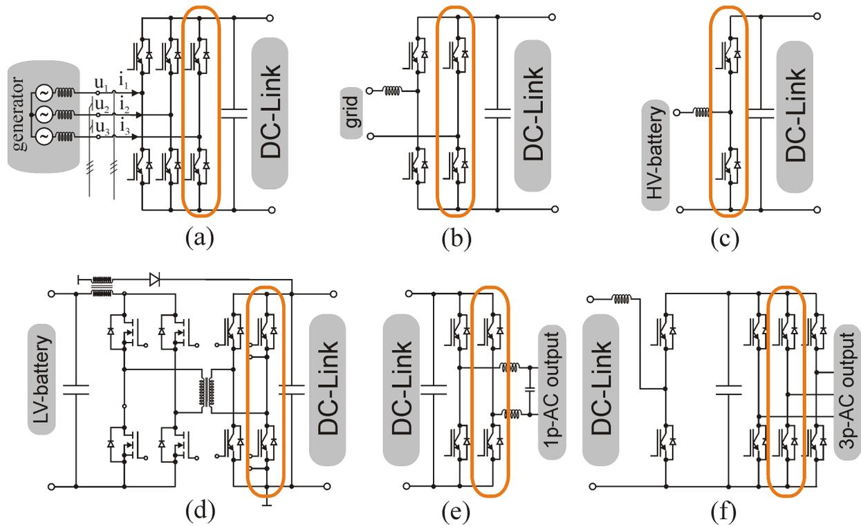
Fig. 2. Converters in system; (a) AC-DC converter-C1, (b) AC-DC converter-C2; (c) DC-DC converter-C3; (d) DC-DC converter-C4; (e) DC-AC converter-C5; (f) DC-AC converter-C6
