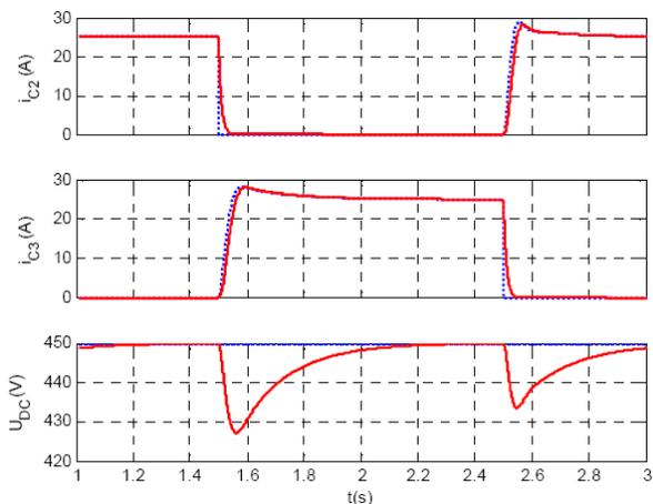
Fig. 18. Transfer from BATTERY mode to ONNET and back from ONNET to BATTERY
