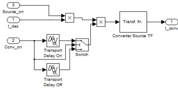
Fig. 6. Model of uni-directional (pure source) converter
