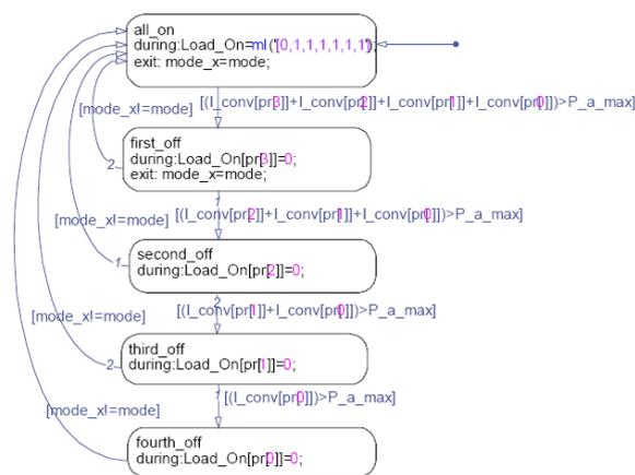
Fig. 13. Stateflow representation of the load management scheme
