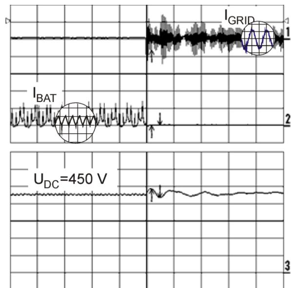
Fig. 15. Transfer from C3 to C2 (1-battery current,  $I_{BAT}$ -5A/div; 2-current to grid,  $I_{GRID}$  5A/div; 3-DC-link voltage,  $U_{DC}$  100 V/div, x-axis 1s/div)
