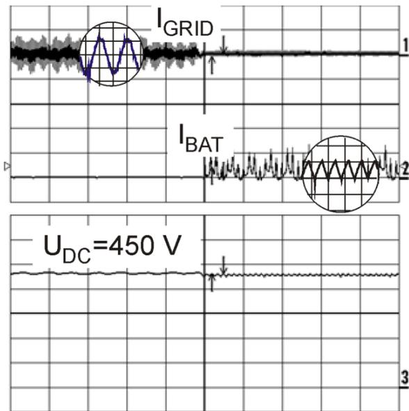
Fig. 16. Transfer from C2 to C3 (1-battery current,  $I_{BAT}$ -5A/div; 2 - current to grid,  $I_{GRID}$ -5A/div; 3- DC-link voltage,  $U_{DC}$ -100 V/div, x-axis 1s/div)
