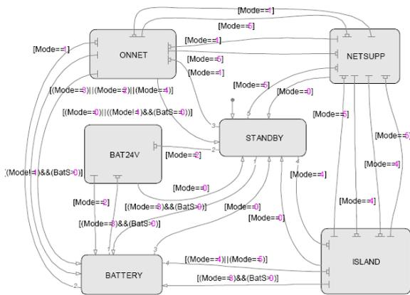
Fig. 11. Stateflow representation of the power management model
