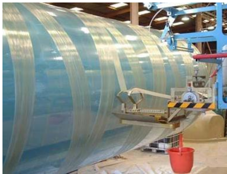
Figure 8. Photo of the composite filament winding machine.
